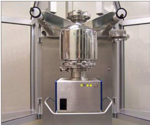
Figure 1: BlendAlyser mounted to a blending system
